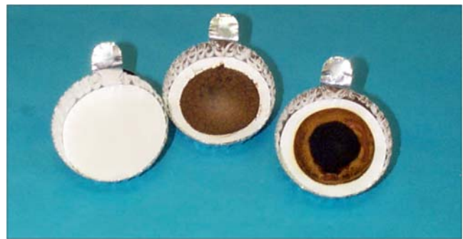
Figure 1. Residue remaining on filter paper (left to right): Calflo AF, A world leader in industrial lubricants, specialty heat transfer fluid competitor.
