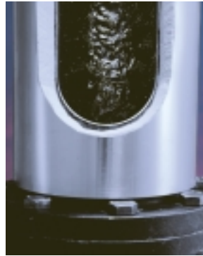
Heavy carbonization of heat transfer fluids.†
